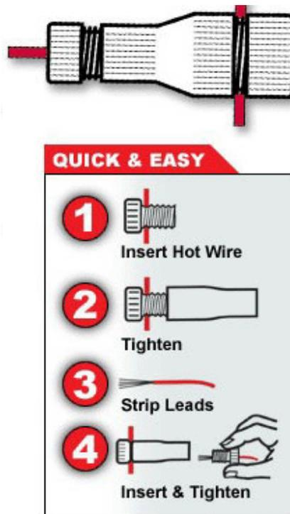
**Scheme 3. How to connect the wires using posi-taps.**
