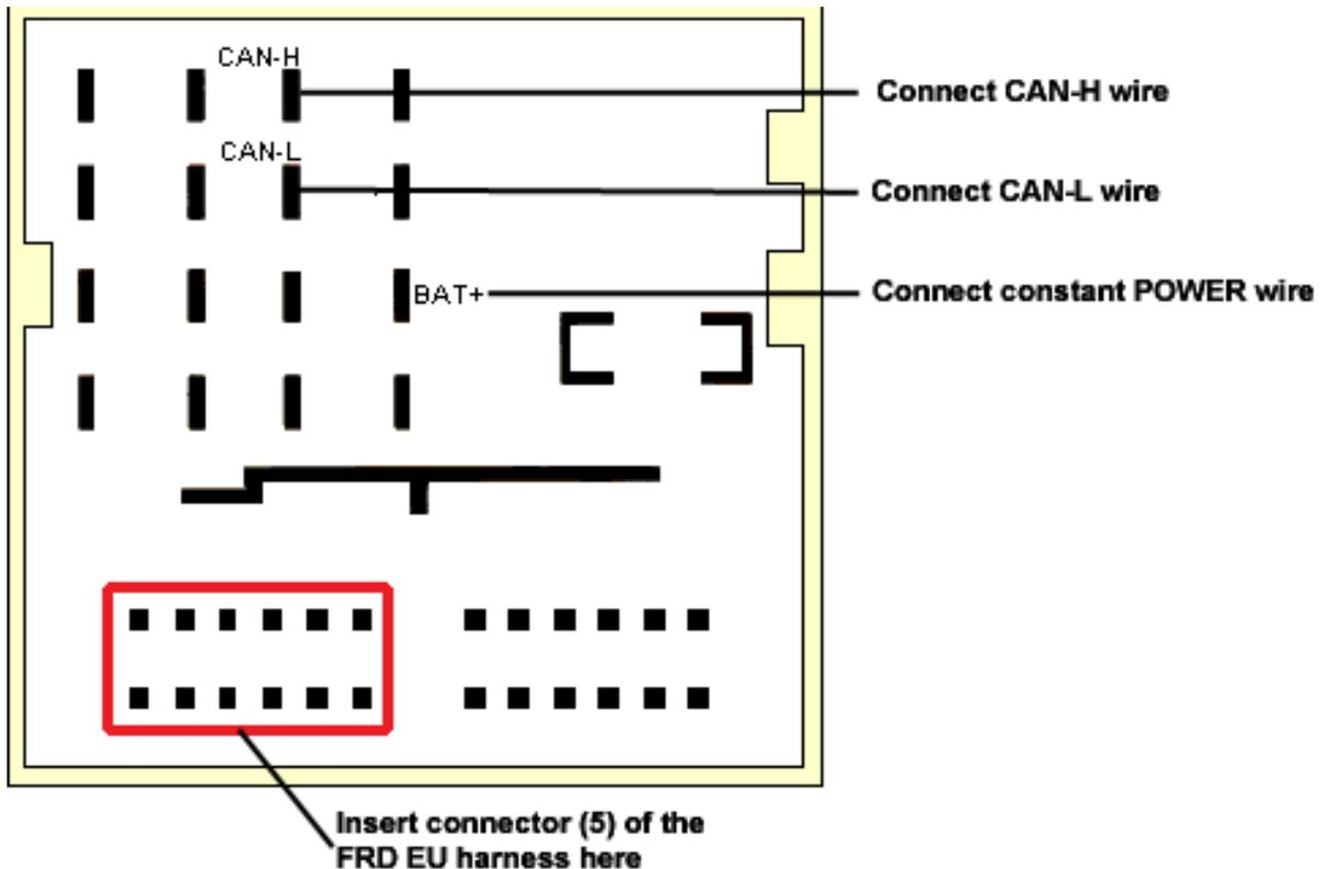
Picture 2: Wiring diagram - main radio harness with CAN-H, CAN-L and BAT+ position
